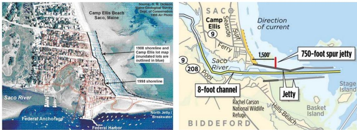
**Figure 1:** 1908-1998 shoreline recession map of Camp Ellis (left) (Dickson, 1995), and schematic of ACOE proposed solution to mitigate erosion rates (right) (ACOE, 2013).
