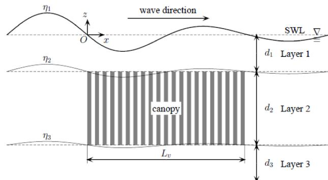
**Figure 2:** Sample schematic of wave attenuation for a three-layer kelp model. SWL is the still water line. The water level surface is given by  $\eta$  and the kelp farm length by  $L_{vp}$  (Zhu et al., 2018).
